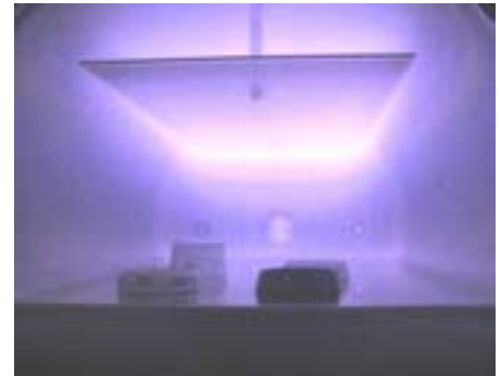
fig. 18 : oxygen plasma, low pressure
