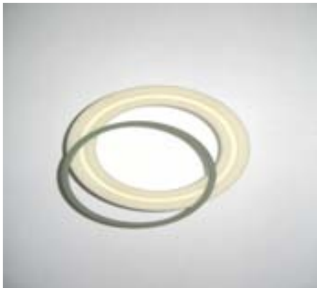
fig. 70: application example of gluing PTFE. treated PTFE is stuck together with a viton ring (Sealing).
